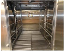
Stainless steel rack washer now completely scale free
