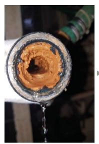
**First inspection: May 21, 2018.**Inside of a secondary small pipe, before Vulcan S25 was installed.
