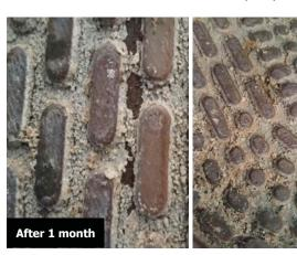
After Vulcan had been installed for 1 month, the scale was softened and falling off.
