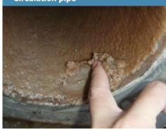
Scale becomes soft and can be easily removed with a finger.
