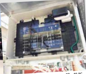
Vulcan S250 outdoor installation: on the roof, with the sun most of the year. The temperature at this time was 38 - 40 °C. In winter, it is rainy and the wrap should be sealed to IP-68. Vulcan impulse bands were well wrapped and the Vulcan unit was in the outdoor box.
