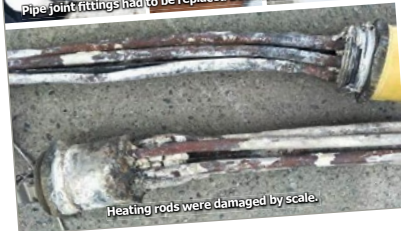
Pipe joint fittings had to be replaced because of scaling and rust.
