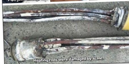
Pipe joint fittings had to be replaced because of scale and rust.
