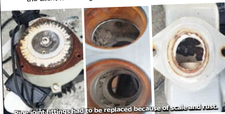
Pipe joint fittings had to be replaced because of scale and rust.
