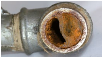
Pipe with limescale deposits
