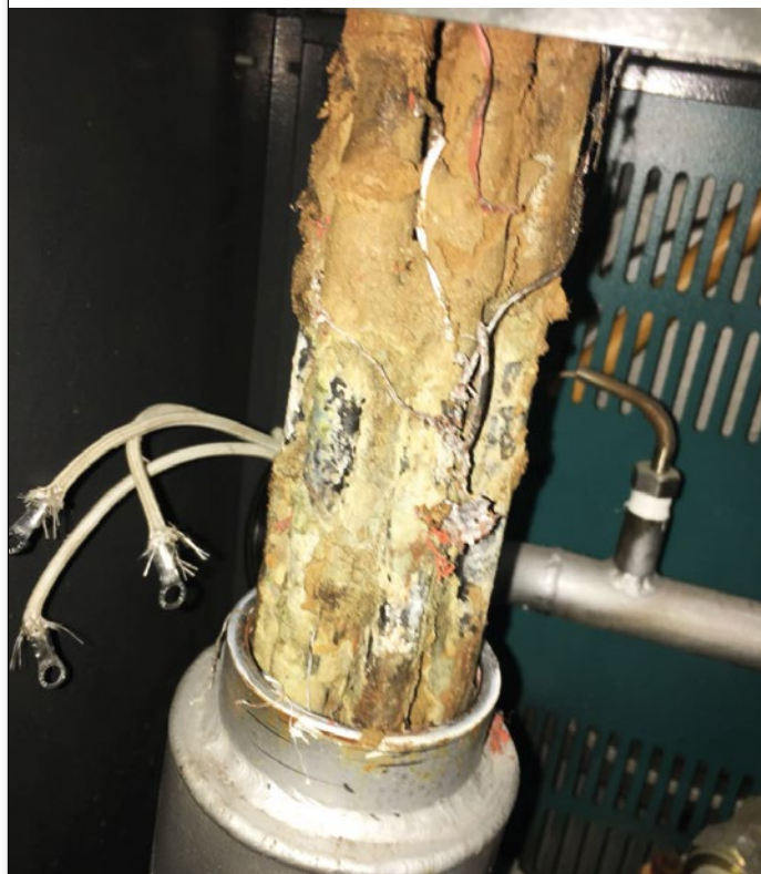
Untreated heat exchanger for 3 years.
