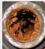
Biofilm in a piping system
