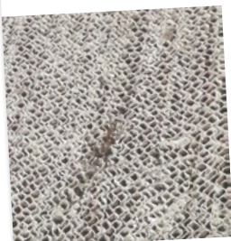
Without any water treatment, the scale was hard like stones, which had not been cleaned for more than 5 years.
